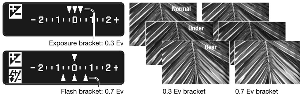
To make a flash bracket, raise the camera flash; the ambient exposure is not bracketed. Only single-frame advance flash brackets can be made regardless of the specified mode; press the shutter-release button for each exposure. The built-in flash recharges between exposures. Exposure brackets are made when the flash is down.
