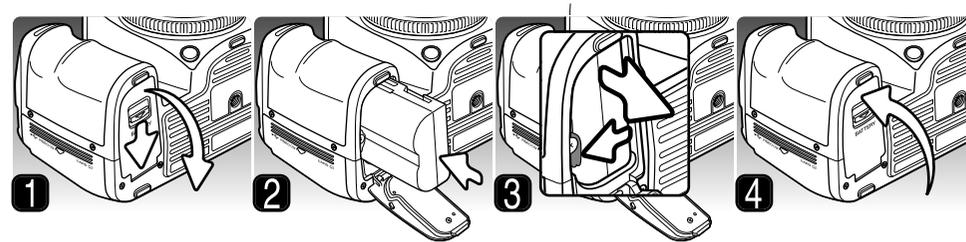
1. Open the battery-chamber door by sliding the battery-chamber release toward the back of the camera.
