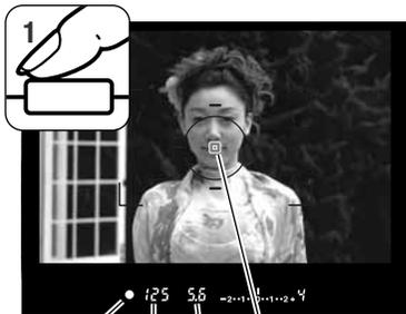
Press the shutter release button partway down to activate the autofocus and autoexposure systems (1). The viewfinder focus signal (A) confirms focus and the spot or local AF area (B) is illuminated briefly to indicate the point of focus. If the focus signal blinks, repeat the procedure.
