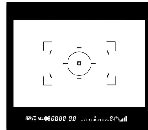
The spot AF area and local focus areas are illuminated briefly to indicate the point of focus when the focus is locked.
