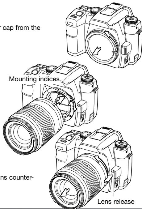
Press the lens release all the way in and turn the lens counter-clockwise until it stops. Carefully remove the lens.
