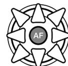
When focus area selection is active, use the controller to select the AF area; autofocus activates and locks each time an area is selected. The central button selects the spot AF area. Focus remains locked after the picture is taken until the controller is released.
