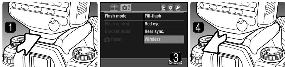
1. Remove the accessory shoe cap (p. 112) and slide a Program 5600HS (D) or 3600HS (D) flash on the accessory shoe until the safety lock engages.
