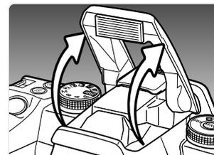
To use the flash, simply pull up the unit by the tabs on each side. The flash position must be set manually, and once up, the flash unit always fires regardless of the amount of ambient light. The flash mode is changed with the recording menu (p. 75).
