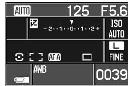
This camera is equipped with an automatic battery-condition indicator. When the camera is on, the indicator appears on the monitor. The indicator changes from white to red when battery power is low. Not all camera functions are available if battery power is low. If the monitor is blank, the battery may be exhausted.
